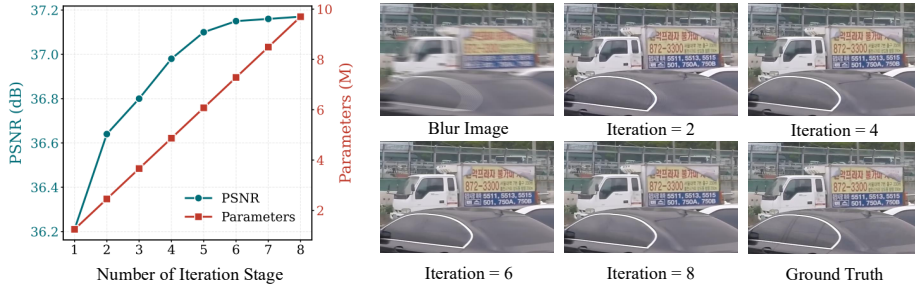
Fig. 7: Effect of the number of unrolled stages N . Left: PSNR and parameter growth with respect to iteration stages. Right: Visual comparisons at different iteration stages.
